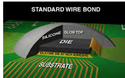
Figure 3. Standard Wire Bond
